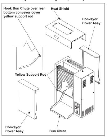
Figure 2. Installing Bun Chute
